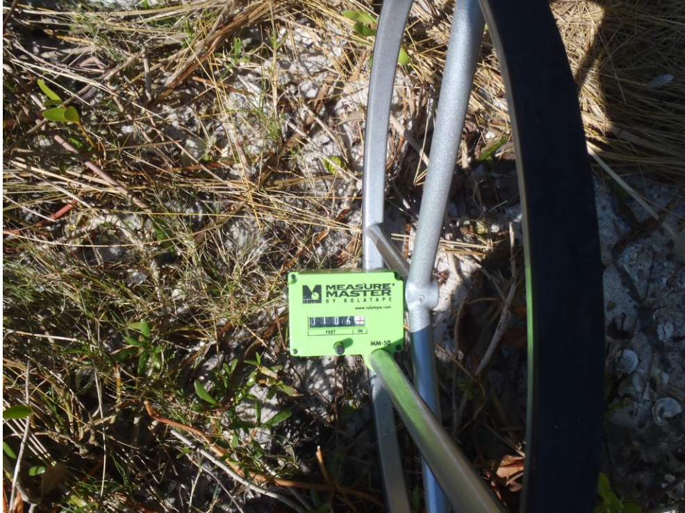
Photo 6: Linear feet of shoreline measured with a wheel.
